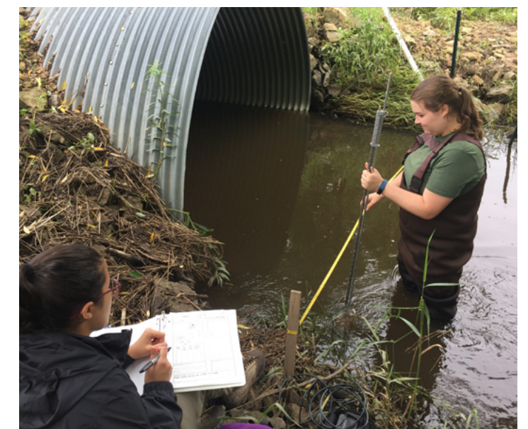
Figure 4.2. Manual flow measurement with a portable flowmeter, recording stream velocity, cross-sectional area, and flow at the Swan@Lalor site. (Photo by Rachel Johnson).
