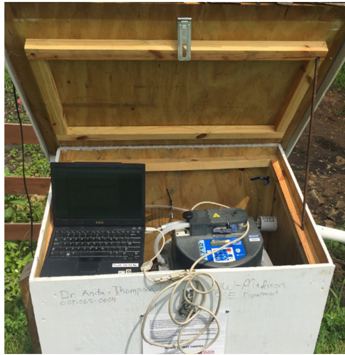
Figure 4.3. Automated sampler monitoring box at the Swan@Lalor site. (Photo by Rachel Johnson).
