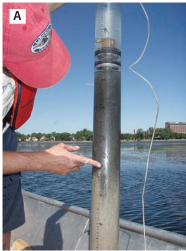
Figure 3.8. A. Sample core taken from Monona Bay showing the transition from pre-settlement marl to post-settlement muck. B. Organic, silty, “contaminated” muck. C. Relatively contaminant-free, calcium carbonate-rich marl.
