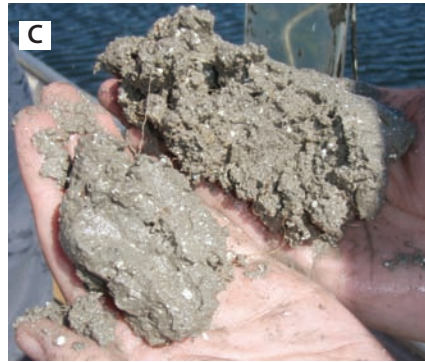
Figure 3.8. A. Sample core taken from Monona Bay showing the transition from pre-settlement marl to post-settlement muck. B. Organic, silty, “contaminated” muck. C. Relatively contaminant-free, calcium carbonate-rich marl.
