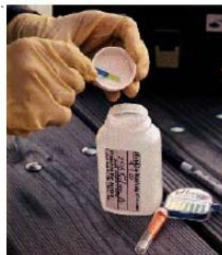
5. Verify sample pH (250 ml bottles). Remove cap from sample bottle and check pH pouring a drop of sample onto the pH paper. Add additional acid if correct pH has not been achieved. Note: No more acid should be needed for lake or river water.
