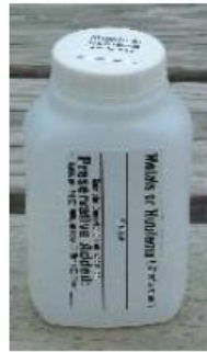
1-250 mL: For nitrogen and Total Phosphorus. Preserve with 1-vial H 2 SO 4 & ice.
