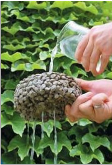
Figure 15.6 An aggregate of pervious concrete used in permeable parking lots, demonstrating the infiltration capability. Source: National Ready Mix Concrete Association. www.nrmca.org
