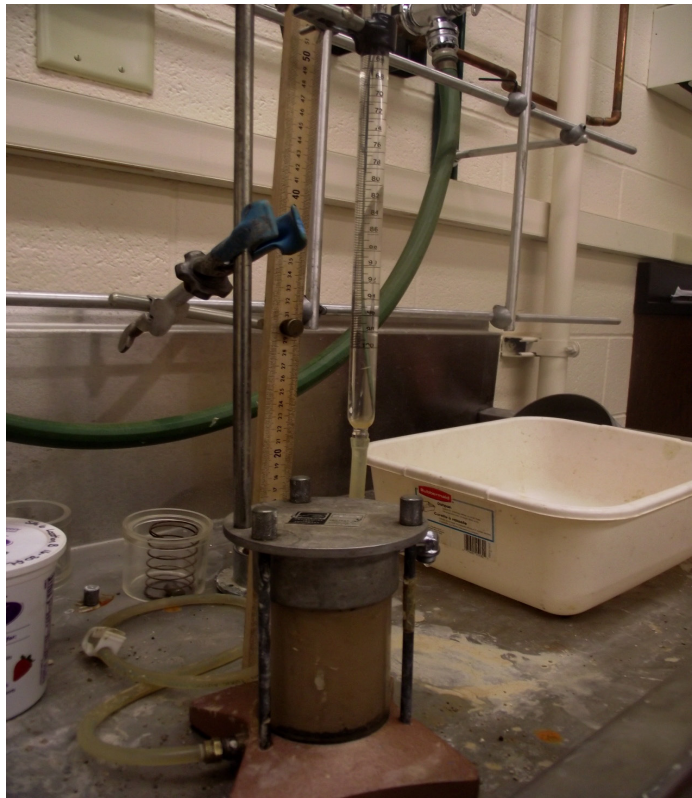
Figure 4.8. Column Test. Two of the sampled soils were used in the shown set-up for column tests.
