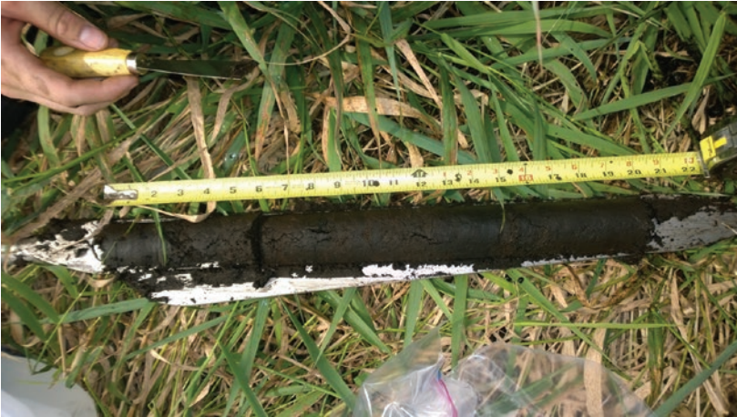
Figure 1.7: Soil sample acquired through a Russian peat borer during the Nine Springs Creek soil analysis.
