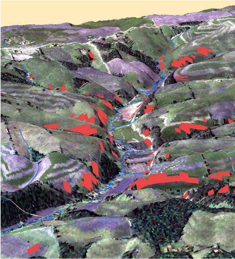
Figure 6.2. An example of how simple and widely available tools and data can be used to show areas (in red) where biophysical conditions are likely to be conducive to excessively high erosion rates if appropriate practices are not in place. (Note: Topography exaggerated for illustration purposes.)
