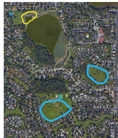
Figure 7.8: Two sites in Madison were selected as candidates for infiltration basins, shown in blue. The location of the proposed forebay is indicated in yellow in the pond's northwest corner.
