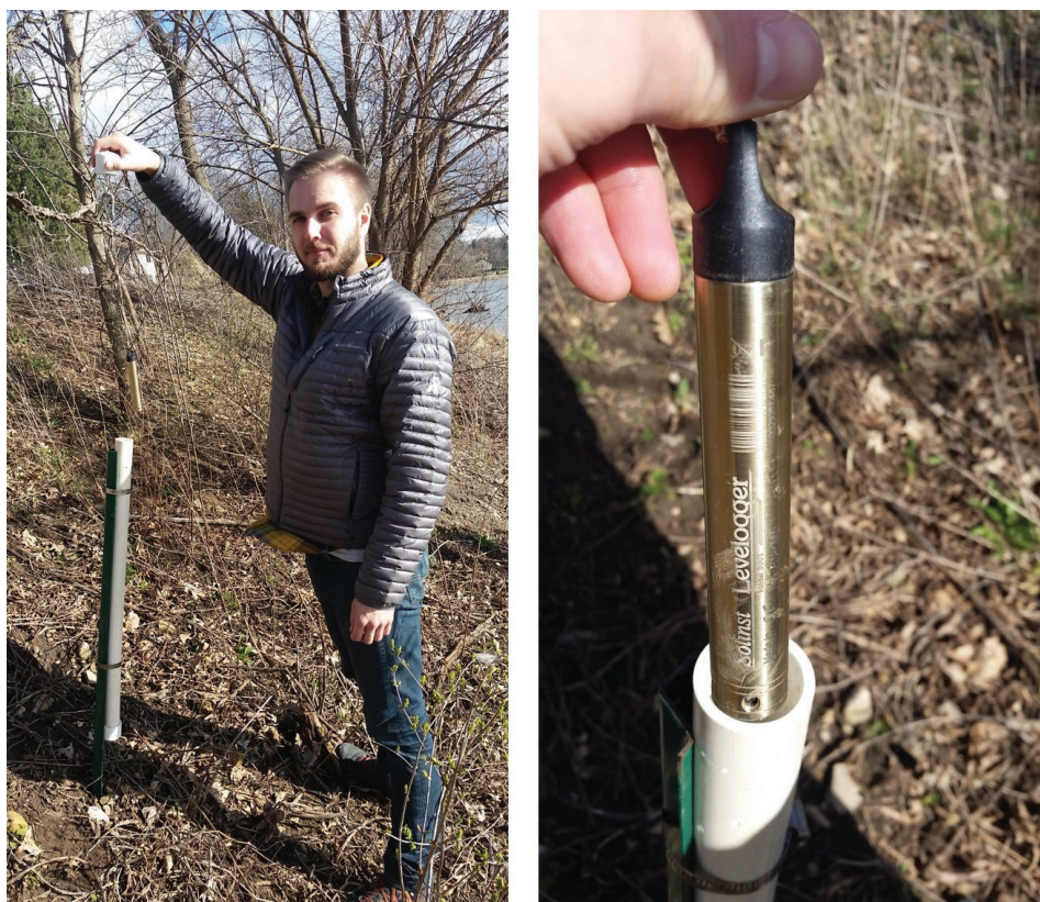
Figure 7.3: Pressure transducers were installed to monitor pond stage and barometric pressure.
