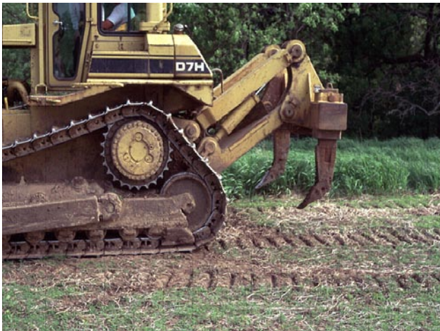
Figure 4.9. Subsoiling, using a dozer, penetrates the surface and can help alleviate soil compaction. Used with permission from A. Roa-Espinoza, Urban Conservationist, Dane County Land Conservation Department (1998).
